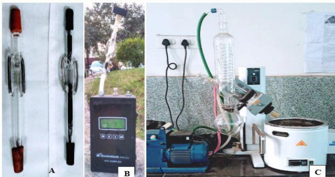
Figure 2.14: [A] Charcoal tube or VOCs sampling tube. Both empty [L.H.S.] and activated charcoal filled [R.H.S.] tubes are shown side by side; [B] VOC sampler and [C] Rotary vacuum evaporator to concentrate the VOC extract in CS 2 solution.
