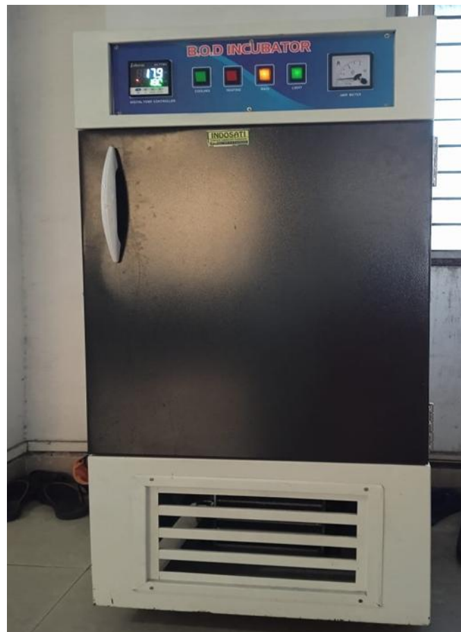
Figure 3.7: BOD incubator used in analysis.
