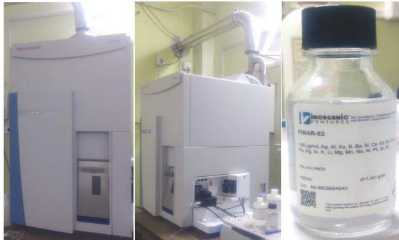
Figure 3.8: ICP-MS with used standard solution [FINAR-92] for instrument internal calibration.
