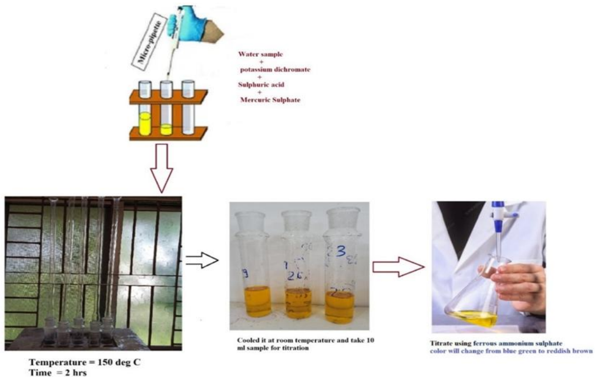
Figure 3.1: Procedure for COD analysis.
