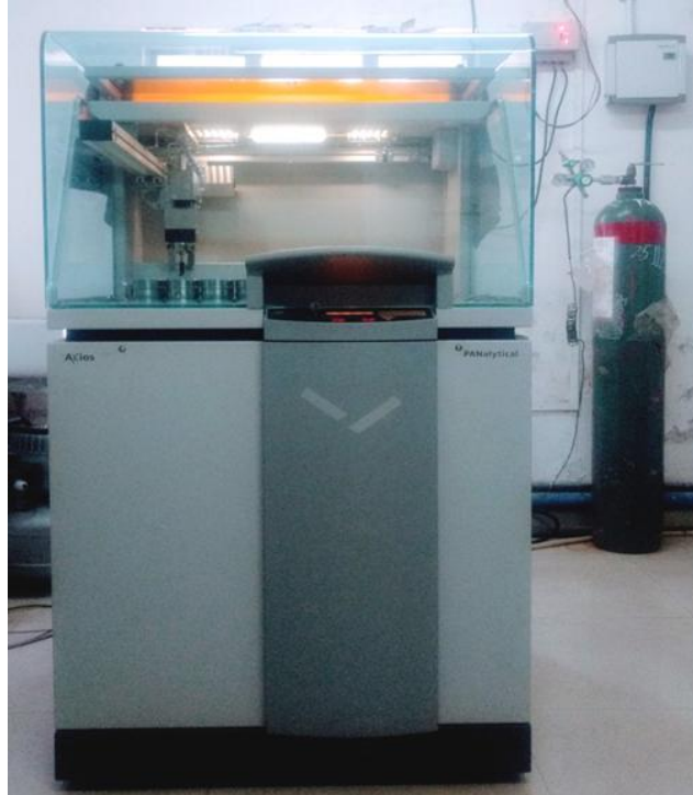
Figure 4.1: X-ray fluorescence spectrometer used for soil analysis.
